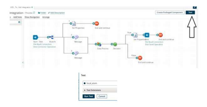
**Step 33:** We see that the process is executed and one file has gone to True shape and the other one to False. Click on disk connector and view the source to see the file which went to disk in the True branch.
